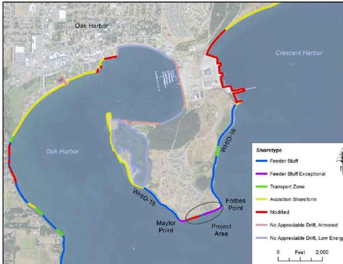
Figure 2. Geomorphic shoretypes of the Maylor Point to Forbes Point area. Note the deteriorated status of some armor resulted in mapping of feeder bluffs where portions of armor remained. (MacLennan et al. 2013)
