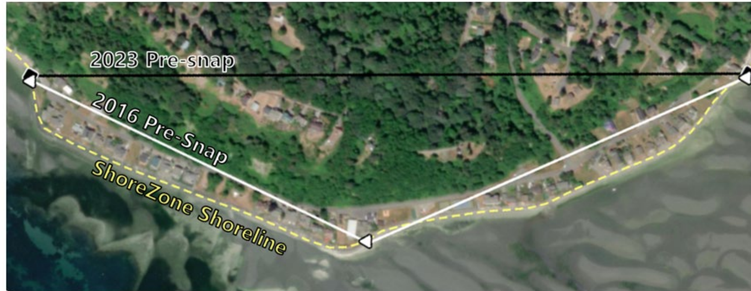
Figure 4. Example of difference in GPS point placement in 2016 and 2023 mapping efforts relative to the ShoreZone Shoreline that produced different pre-snap shoreline armor measurement results.
