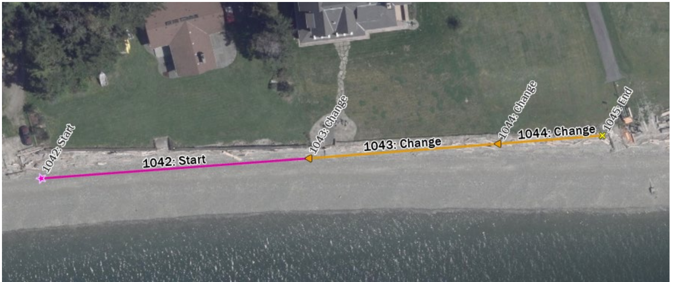
Figure 3. Example of Armor Lines Generated Using Sequentially Assigned Identifiers, with Attributes Populated from Start to End.
