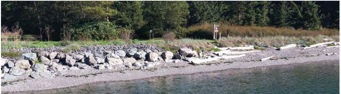
Figure 8. Hard protection measures (left) and soft protection (right) on neighboring Washington beachfront properties.
