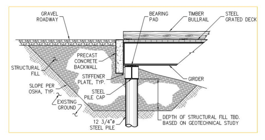
• Option 3 - A fully steel option which could be advantageous if concrete costs escalate or there is no other cast-in-place concrete utilized on the project.
