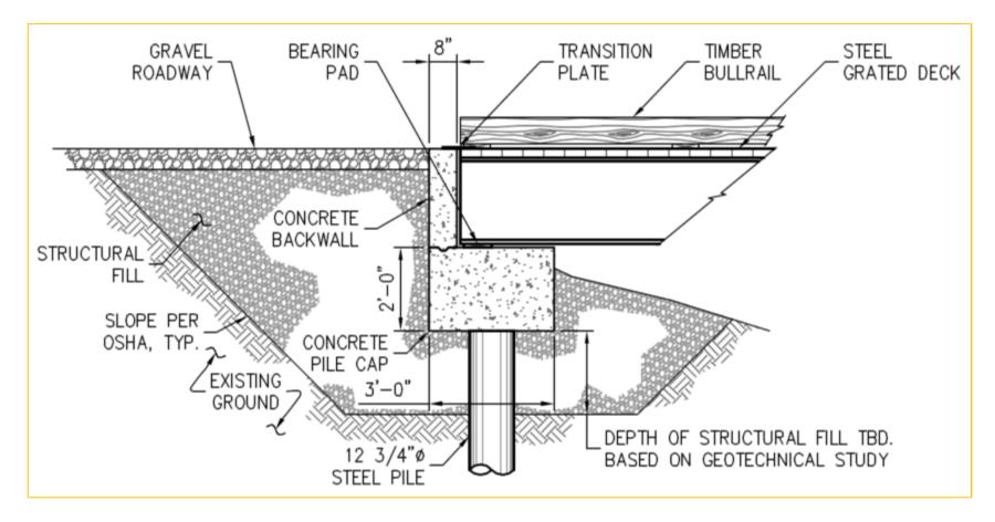
• Option 2 is similar to the standard spread footing with a pile-supported foundation. This more complex option will be required if soft soils are encountered.
